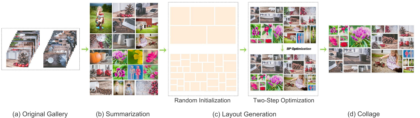
Fig. 2. Workflow of our visual summarization pipeline. Given an input image collection. (a) we first make a representative summary. (b) The output collage is randomly initialized and then refined by optimization. (c) We show the final visual summary in (d).
